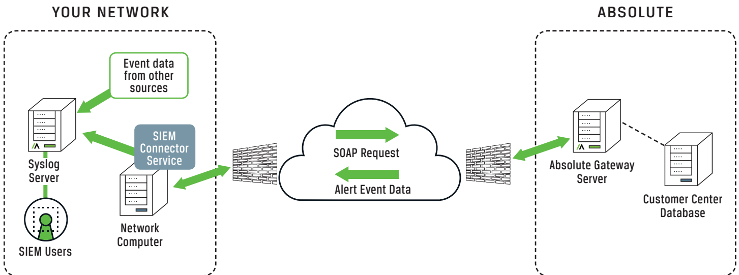
Figure 1: SIEM integration using Absolute SIEM Connector
